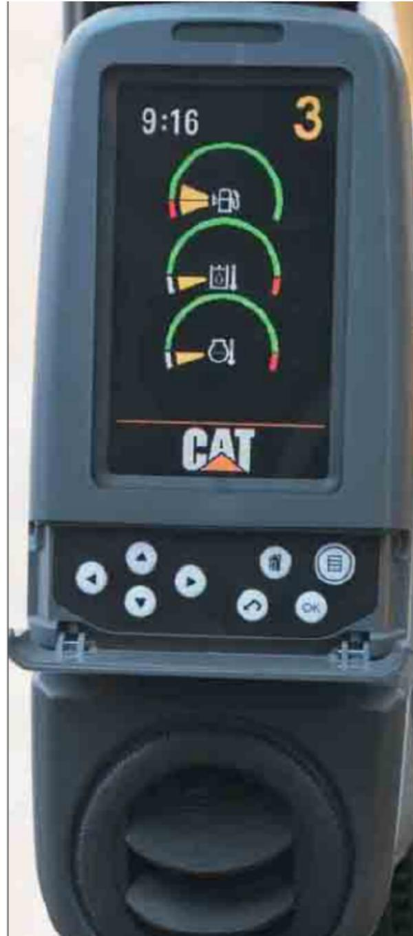
**Monitor Display Screen.** The monitor is a full color 400x234 pixels Liquid Crystal Display (LCD) graphic display. The Master Caution Lamp blinks ON and OFF when one of the critical conditions below occurs:
