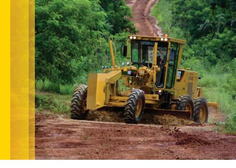
The K Series Motor Grader is the machine you can count on when you need to get work done. Cat® motor graders help you make the most of your investment by delivering maximum productivity and durability. The Cat C7 ACERT™ engine, direct-drive power shift transmission and load sensing hydraulics work together to ensure the power and precision you need to work in demanding conditions. And Cat motor graders are backed by the world-class Cat dealer network to keep you up and running.
